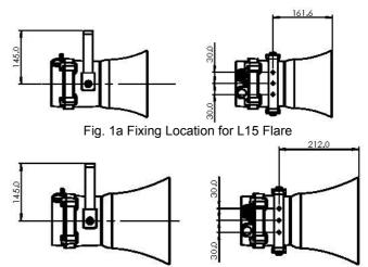
Fig. 1b Fixing Location for L25 Flare
