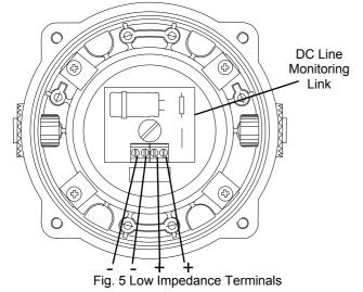
BExL15D 8 $\Omega$  and 16 $\Omega$  low impedance loudspeakers have dual input terminals on the pcb assembly for input and output wiring. A cable of up to 2.5mm<sup>2</sup> can be connected to each terminal. If dc line monitoring is used cut the link on the board (see figure 5 and section 14 of this manual).
