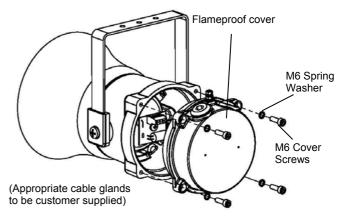
Fig. 2 Accessing the Explosion proof Enclosure.
