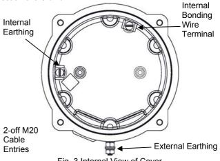
Fig. 3 Internal View of Cover
